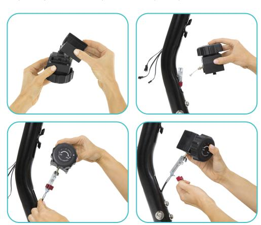
15. Fit Tension knob into center rectangular whole. Position the Tensioner Cap on the backside of the Handlebar Post opposite the Tensioner, and secure in place with the Small Flat Washer and the Long Phillips Screw.
